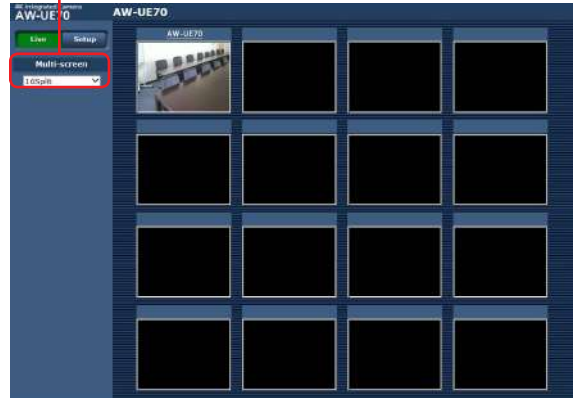
Multi screen consisting of 16 sub-screens
