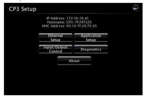
The "CP3 Setup" menu displays the IP address, hostname and MAC address of the device. It also allows access to various setup and programming screens. The "CP3 Setup" menu contains buttons for **Ethernet Setup**, **Application Setup**, **Input/Output Control**, **Diagnostics**, and **About**, as shown in the illustration above.
