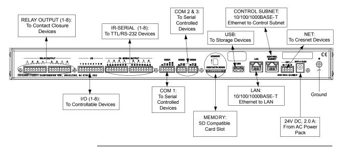
**NOTE:** Ensure the unit is properly grounded by connecting the chassis ground lug to an earth ground (building steel).
