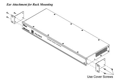
4. Repeat procedure (steps 1 through 3) to attach the remaining ear to the opposite side.
