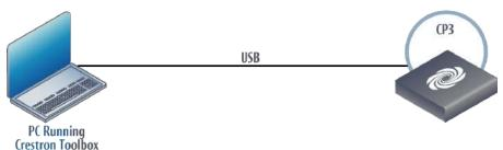
The **COMPUTER** port on the CP3 connects to the USB port on the PC via the included Type A to Type B USB cable:
