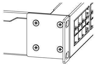
3. Tighten screws to secure it in place.
